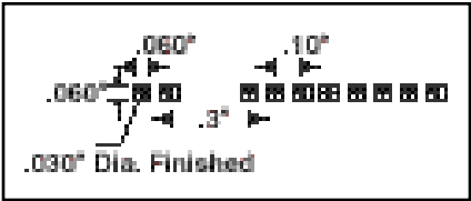
figure 6: Recommended PCB footprint
